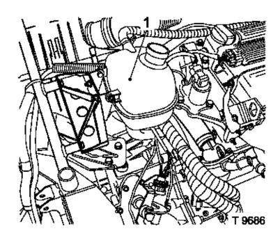
Oil pipe (1) from the oil filter housing.
