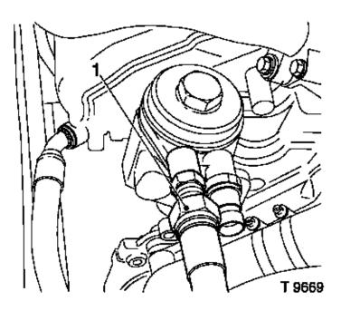
Expansion tank (1) to the bracket – bolts.
